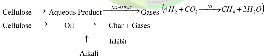
Fig. 1. Reaction path way for the hydrothermal liquefaction of cellulose.
