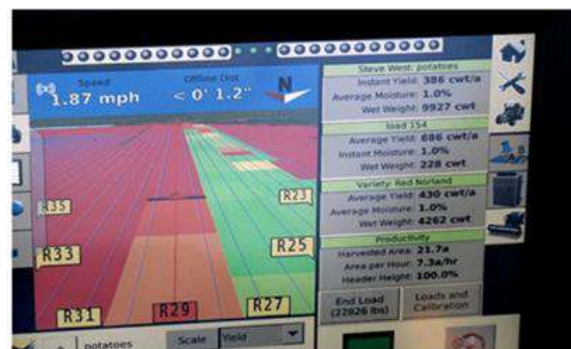
Fig- processing of yield data into yield maps using computer based software
