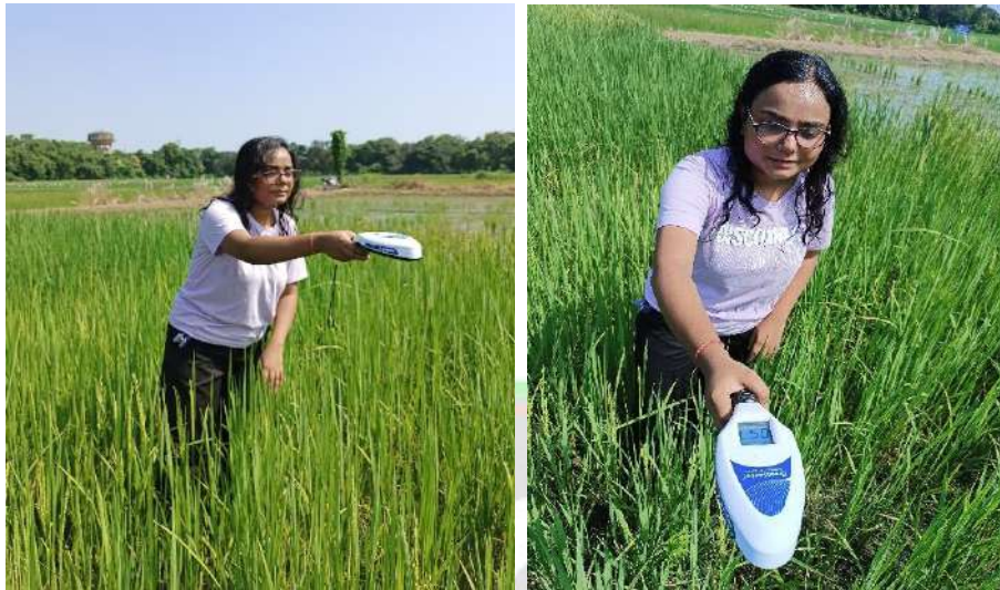
Taking NDVI value of paddy field (80 days after planting) at B.H.U., Varanasi
