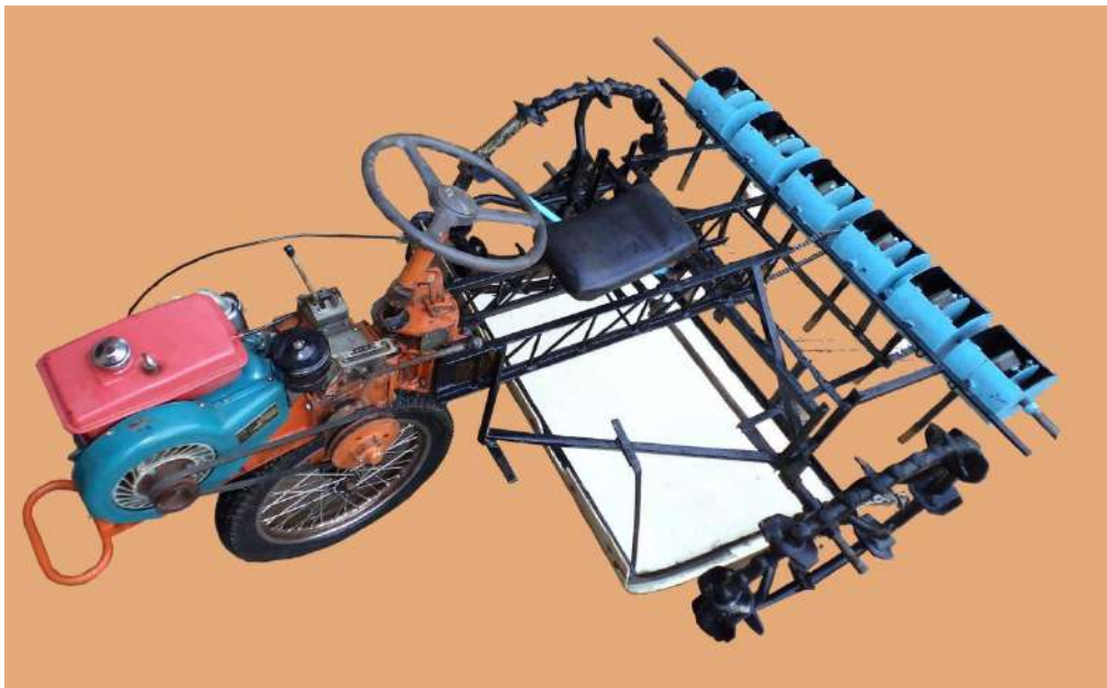
Plate 1 Idle view of the self-propelled lowland rice seeder
