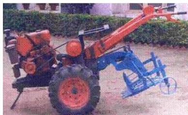
Power tiller operated turmeric harvester
