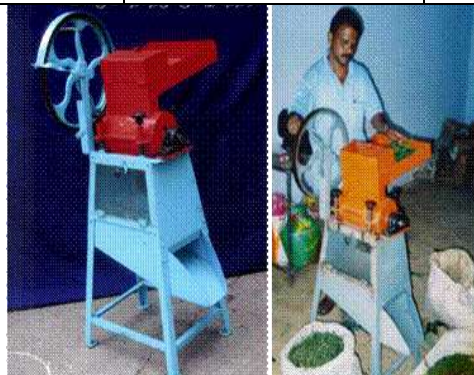
Hand operated pepper thresher developed by TNAU
