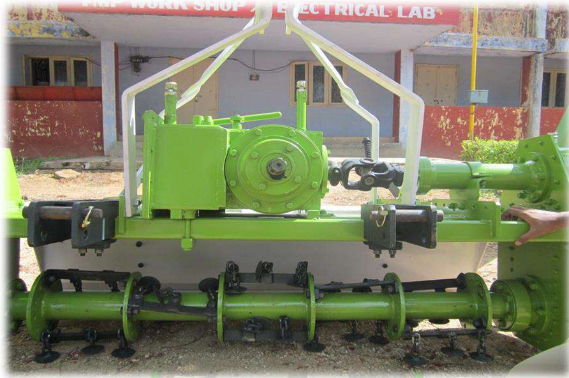
Plate 1. View of the Rotavator cum flail mower
