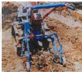
Power tiller operated turmeric harvester
